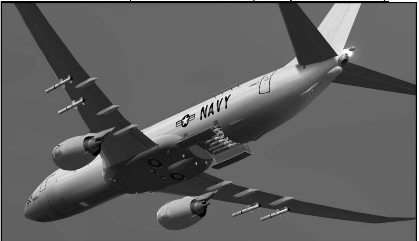
ABOVE: Boeing artwork showing a P-8’s hard points loaded with Harpoon missiles and its bomb bay full of torpedoes and other ordnance.
