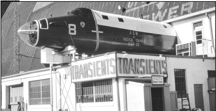
**ABOVE:** Remember the GSP-2E? This was the forward fuselage section of an SP-2E that had an engine fire on the ground at NAS Brunswick. It was trucked to NAS South Weymouth and mounted on top of the south lean-to on the side of Hangar One, wired up to simulation equipment in the ASW Training Department's spaces, and was used as a tactical trainer for many years. Photo by Richard Sullivan courtesy of Stephen Miller. Got something similar to share? If so, contact Marc J. Frattasio.
