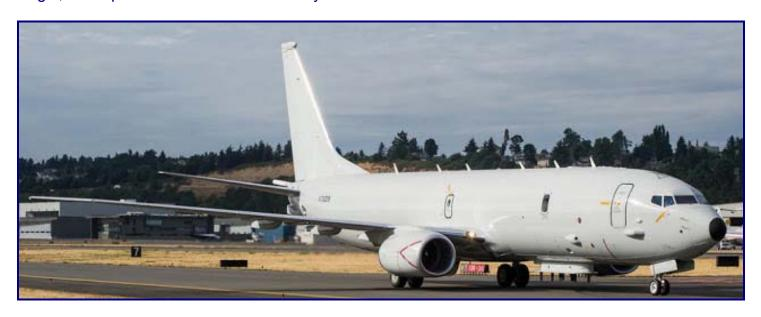
**ABOVE:** P-8 Poseidon at Boeing Field in Seattle, WA. Note the unusual antenna array mounted under forward fuselage between wing and cabin door. Josh Kaiser photo, Defence Blog.
