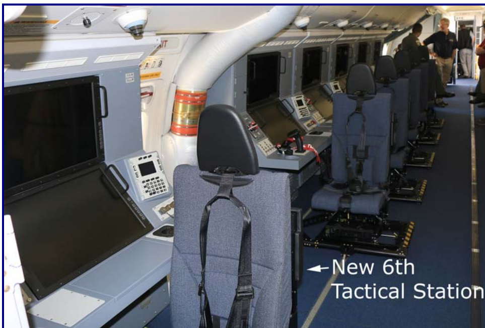
ABOVE LEFT: Interior view of P-8A tactical crew stations. ABOVE RIGHT: Updated P-3C acoustic sensor stations with new center monitor.
